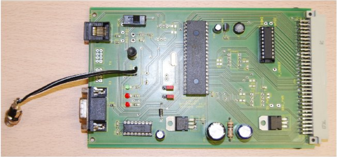
Figure 2: Microprocessor board for the power supply and I/O's ports.
