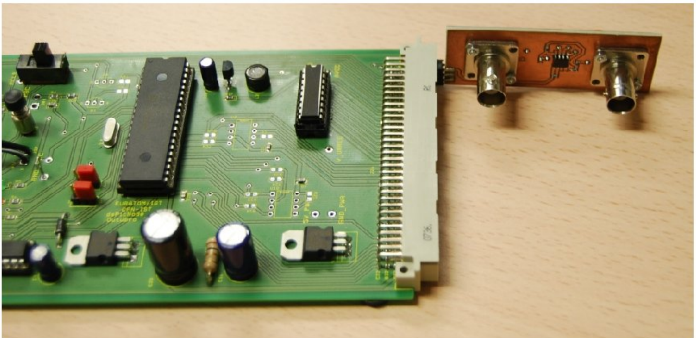
Figure 7: Signal conditioning board connected to the microprocessor board.
